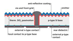
Schematic cross section of a p-type highperformance MWT (HIP-MWT) solar cell, which only demands one additional process step compared to passivated H-pattern cells.
