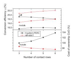
Evaluation of conversion efficiency and cost of ownership of screen printed HIP-MWT and H-pattern PERC solar cells and modules fabricated in Europe. All cells exhibit 9 solder pads per contact row. The finger witdh is reduced subsequently from 60 µm (3 BB) down to 45 µm (6 BB). The busbar width for H-pattern is 1.5 mm for all metallization layouts.
