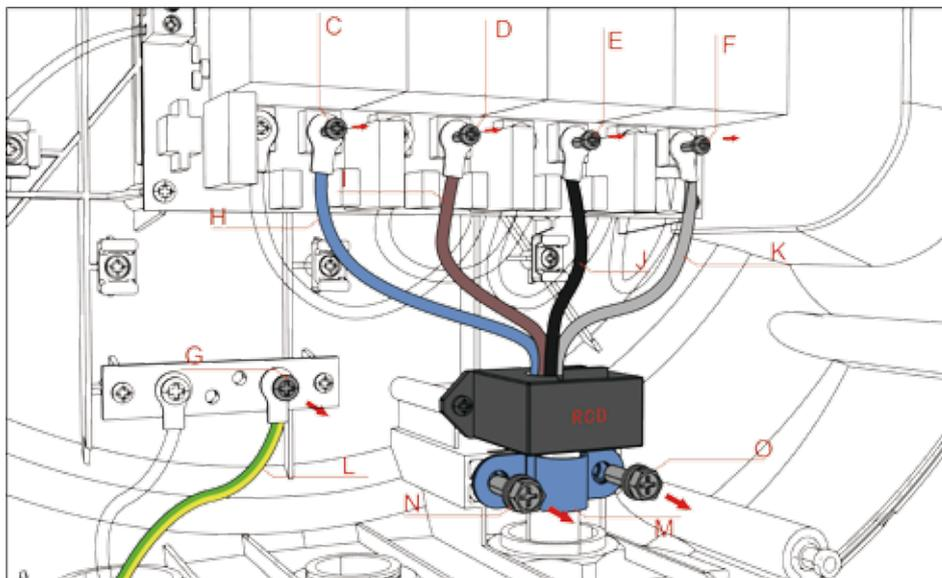
4) Unscrew screws N and O which are used to fix hose clamp M
