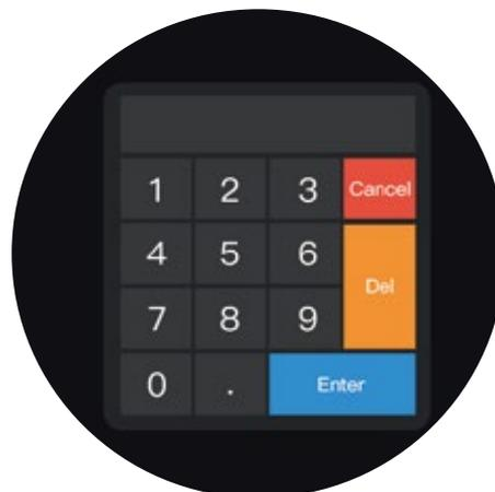
Tap the Set Time button and the numeric keypad will show up. Enter the correct time in the sequence of year, month, day, hour, minute and second (yyyy-MM-dd-HH-mm-ss). Please note that dots should be entered between each data.
